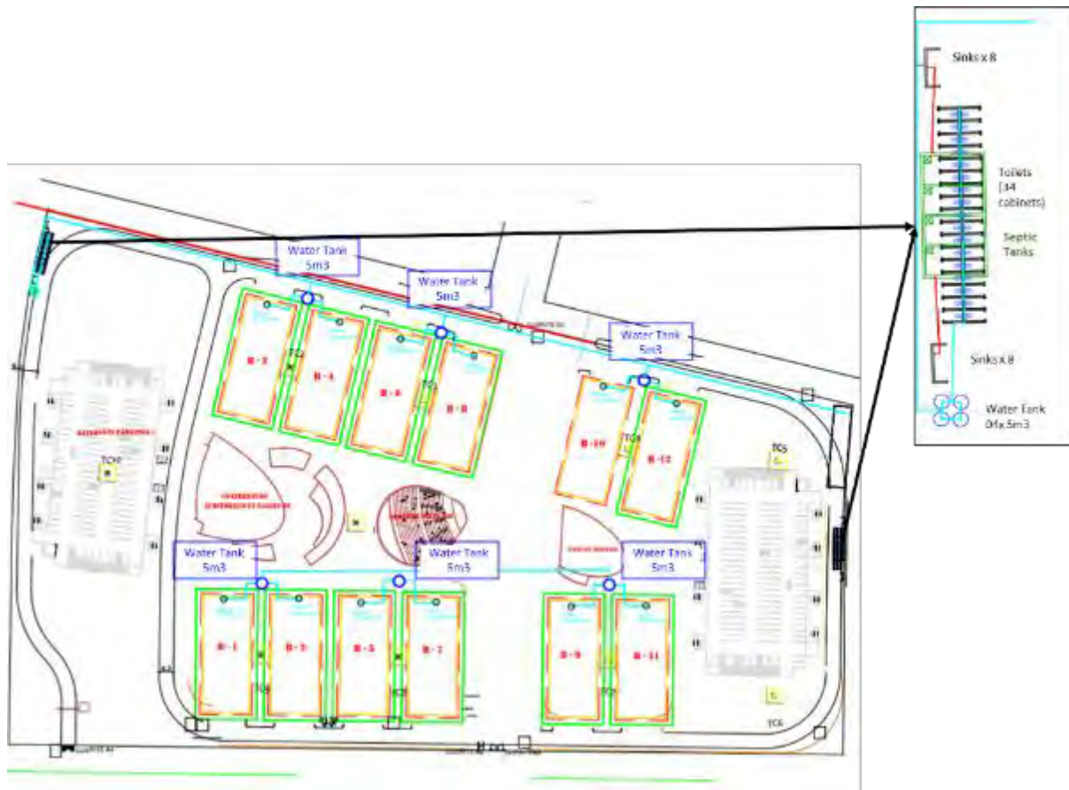
Figure 2-9: Site Drainage Plan (Toilet cabinets, septic tanks and the location of the water tanks are also indicated in the figure)
